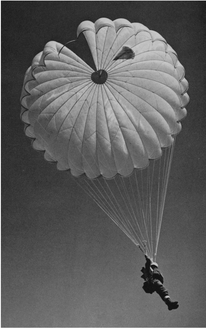
12. Original GQ Single Blank canopy in freefall mode. Note position of the blank gore.
