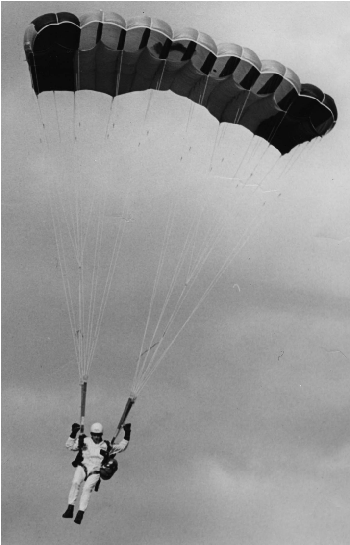
78. The author on Mk 1 Paraplane, February 1973. Note no stabiliser panels, no slider.
